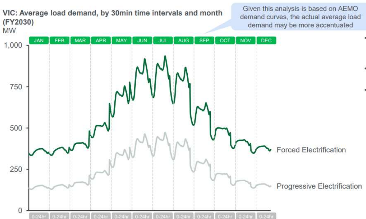
Figure 7 - Extract from LEK. Consulting report - Victorian average load demand as a result of the RIS
